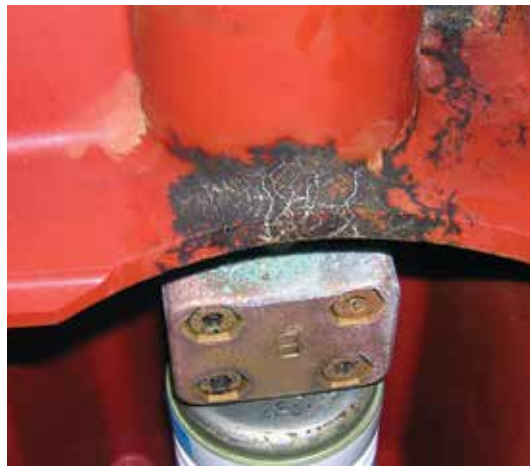
Figure 5: Effects of Unmitigated Partial Discharge in Insulation
