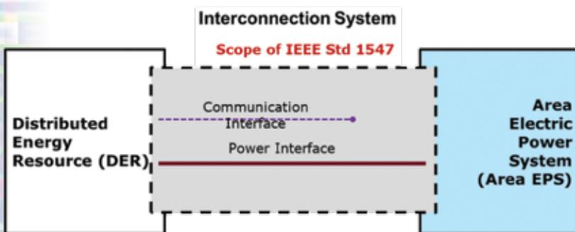
Figure 3: Diagram of Interconnection System
