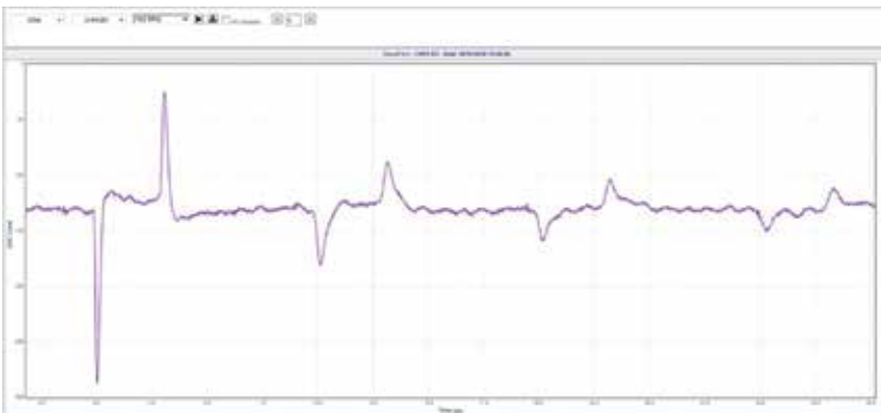
Figure 4: PD Current Pulse Recorded on CHP2-R2
