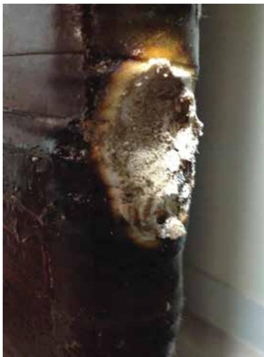
**Figure 3:** *Close-Up of Damage on Edge of Busbar*
