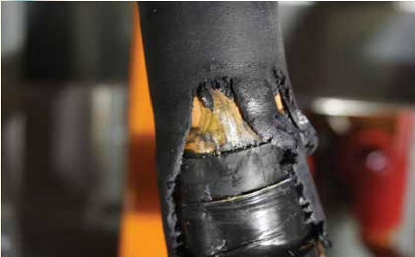
**Figure 4:** *Damaged Cable Termination*
