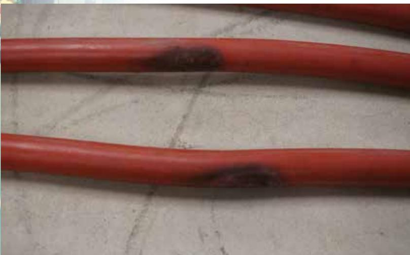
**Figure 6:** *Damaged PT Cables*
