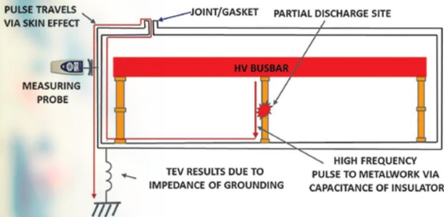
**Figure 1:** *Current Flow Resulting in Transient Earth Voltage*
