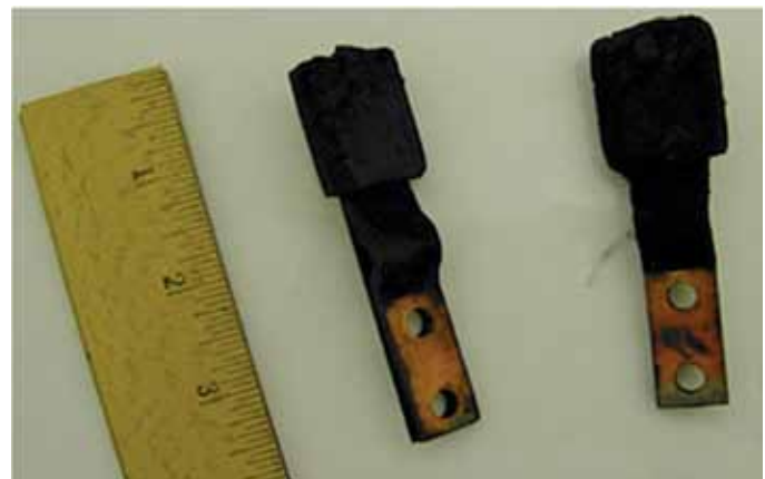
Illustration 1: Burned reversing switch contacts
