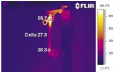
Figure 2 — Correct focus produces good measurements and looks professional. Simulated hot spot problem from the Infrared Training Center IR camera laboratory.
