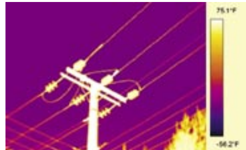
Figure 7— Poorly thermally tuned for finding problems.
