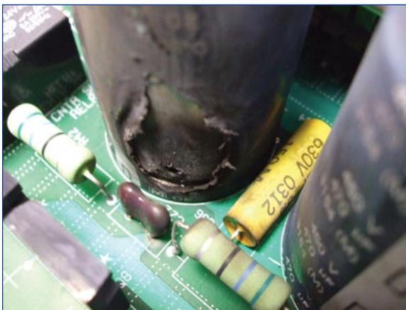
Photo 2—Random component failure
