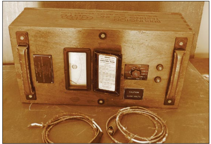
Figure 4 — The Megger Series 1 insulation test kit was a sturdy, reliable instrument.
