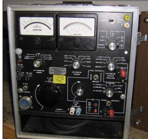
Figure 1 — The equipment used in relay testing has evolved drastically in the past 25 years to keep up with the changing relay itself.
