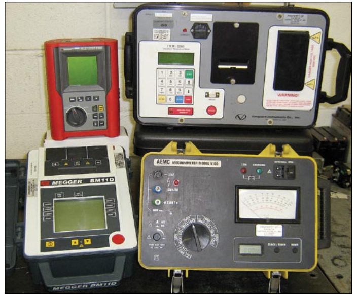
Figure 5: — Today's insulation resistance test sets are truly portable and offer a variety of result outputs.
