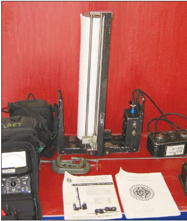
Figure 2 — This circuit breaker operation analyzer was applicable to all breakers of the time period except for those having rotary motion of the contacts.
