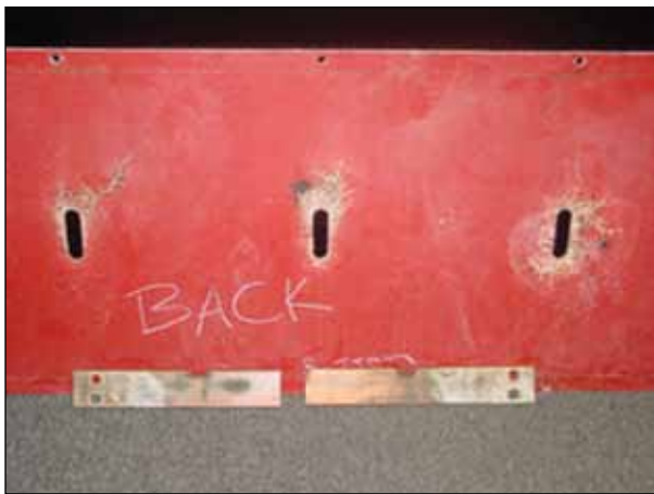
Figure 3 — Switchgear Bus Support Barrier
